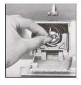
Hold the bobbin case by the latch with the index finger and thumb of the left hand. Insert so that the finger of the bobbin case points upwards, engaging in the notch of the hook race cover. Check: Pull end of thread. Close the hinged front cover.
