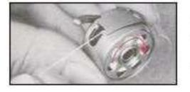
When the end of the thread is pulled, the bobbin should turn clockwise, in the direction of the arrow.
