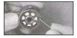
Take the thread anticlockwise to the slot.
